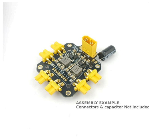
Figure 5: Example assembly with XT60, XT30 connectors and external input capacitor installed. Connectors and capacitor not included.
